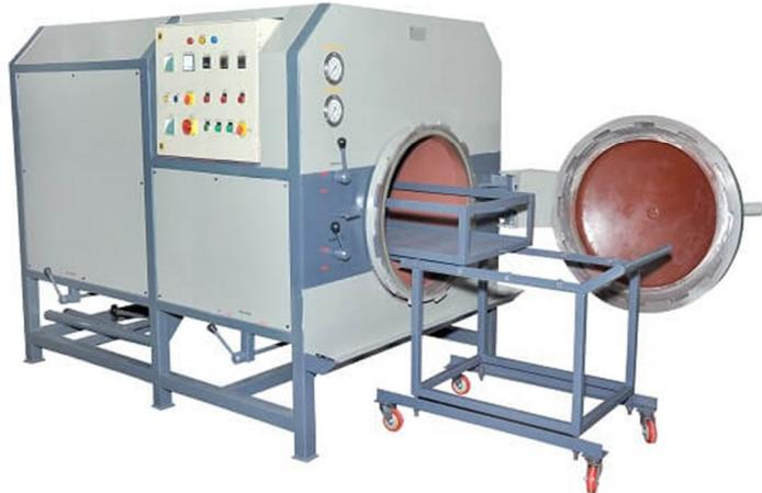
After the shell building procedure is complete, the wax within the wax within monolithic shell is removed. The de-wax autoclave quickly and efficiently melts out the wax from the shells. The autoclave de-wax is the most reliable and cost effective process for large production runs.
